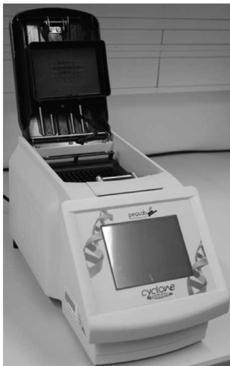
Fig. 13.2 PCR machine, also known as a thermal cycler.
